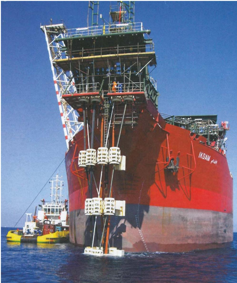
**Figure 1.** TCMS production tower on the Ikdam project offshore Tunisia, showing three risers and two umbilicals.
