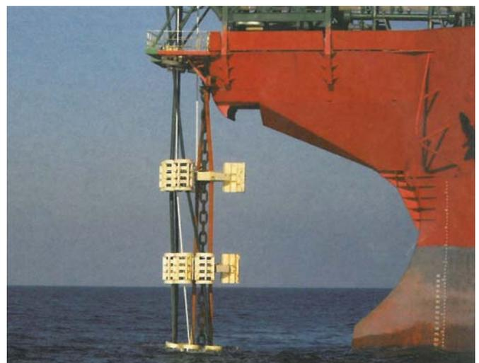
*Figure 3. TCMS production tower showing chafe chain, guide collars, risers and umbilical.*
